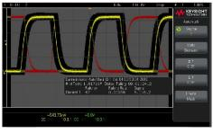
1000 X-Series' hardware-based mask testing can quickly validate a signal's quality and detect errors with up to 50,000 tests per second. Standard on DSOX models
