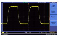
With the infinite persistence display mode turned on, the TBS1000B never sees the glitch after 90 seconds. This is due to its slow update rate of 100 wfms/s.
