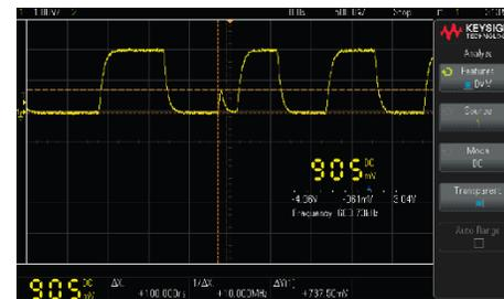
Integrated digital voltmeter (DVM) allows you to characterize signals independent of the oscilloscope's triggering system.
