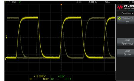
With the infinite persistence display mode turned on, an infrequent glitch is captured after 2 seconds on the 1000 X-Series with 50,000 wfms/s.
