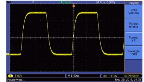
With the infinite persistence display mode turned on, the TBS1000B never sees the glitch after 90 seconds. This is due to its slow update rate of 100 wfms/s.
