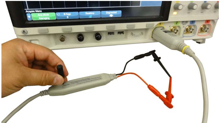
Figure 7 Adjusting the Offset Using the Supplied Tool
