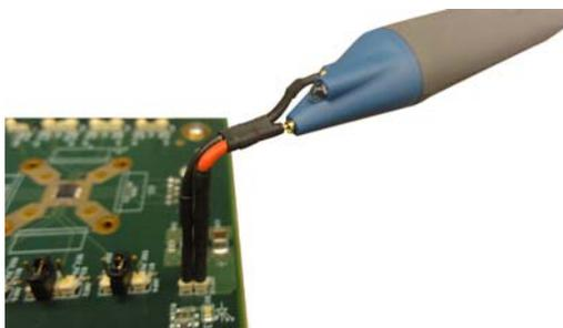
**Figure 5 Probe with Y-Leads Attached**
