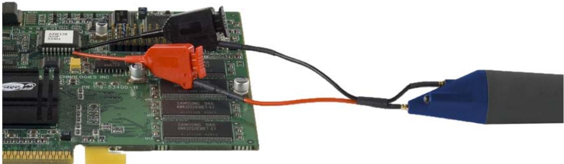
**Figure 8** Probe with Flexible Nose Clips Attached
