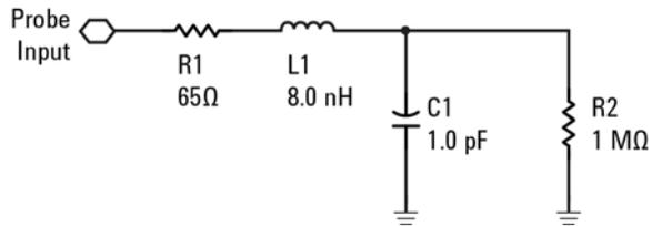
**Figure 13** Input Impedance Equivalent Model
