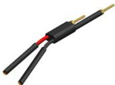
The short 6 cm long Y-leads offer a convenient and reliable method to connect both the probe signal and ground to probe points on the board via or the solderable pins that are provided with each probe. The sockets accept 0.56 to 0.86 mm round and 0.64 mm square (0.022 to 0.034 inch round and 0.025 inch square) diameter pins. The maximum insertion depth is 7.5 mm (0.295 inch) and the outer insulation of the socket is less than 2.54 mm. You can use it for 2.54 mm pitch (0.1 inch) terminals.
