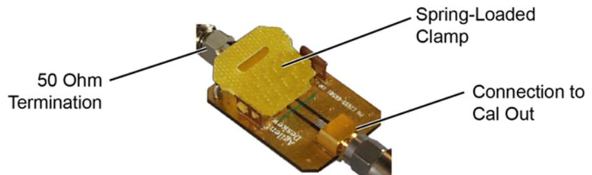
**Figure 10 E2655B PV Fixture with 50 Ohm Termination**
