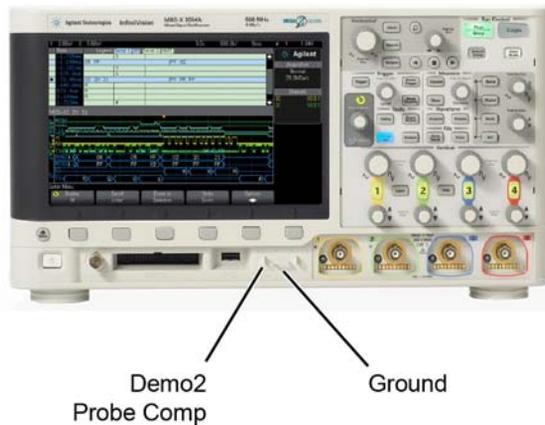
**Figure 11 Probe Calibration Terminals on 3000 X-Series Oscilloscope**
