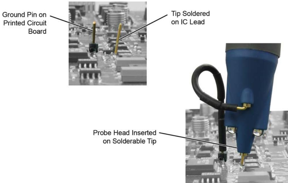
**Figure 6** Placing the Probe Onto the Solderable Tip
