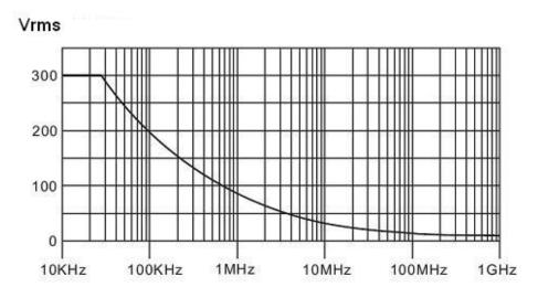
Figure 4. Voltage derating curve
