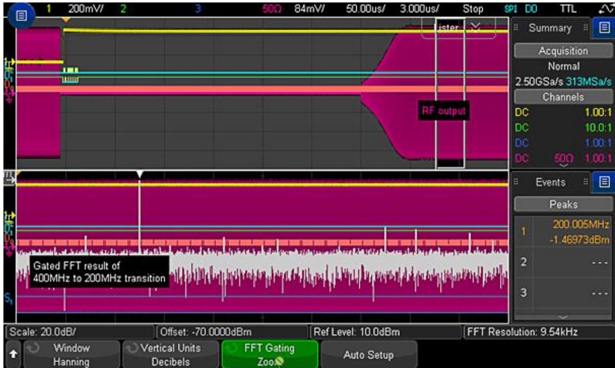
Figure 24. RF signal settled down at 200 MHz as indicated in the search lister.
