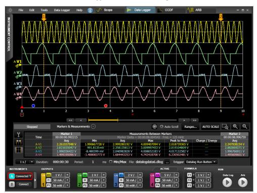
Select the Data Logger button from the top of the window.
