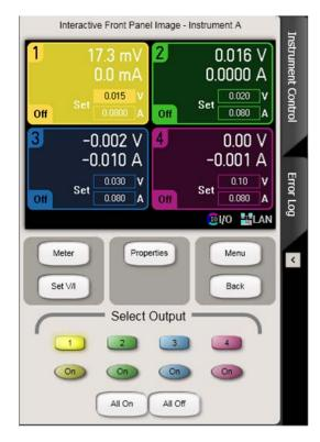
**Meter** - Displays the meter view. Toggles between single output and multiple output views.
