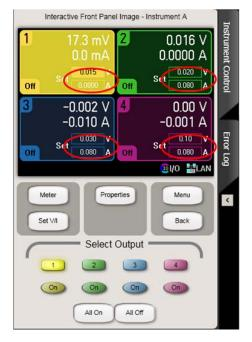
Step 2. Click the Source Settings button twice. In the Output On/Off Delay area, configure the output turn-on sequence as follows. You will only need to configure the Turn-on delays, not the Turnoff delays.
