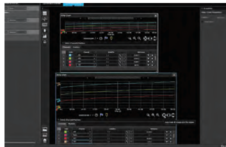
Figure 3. To view your logged data, set up a strip chart to display the temperature measurements on each channel.
