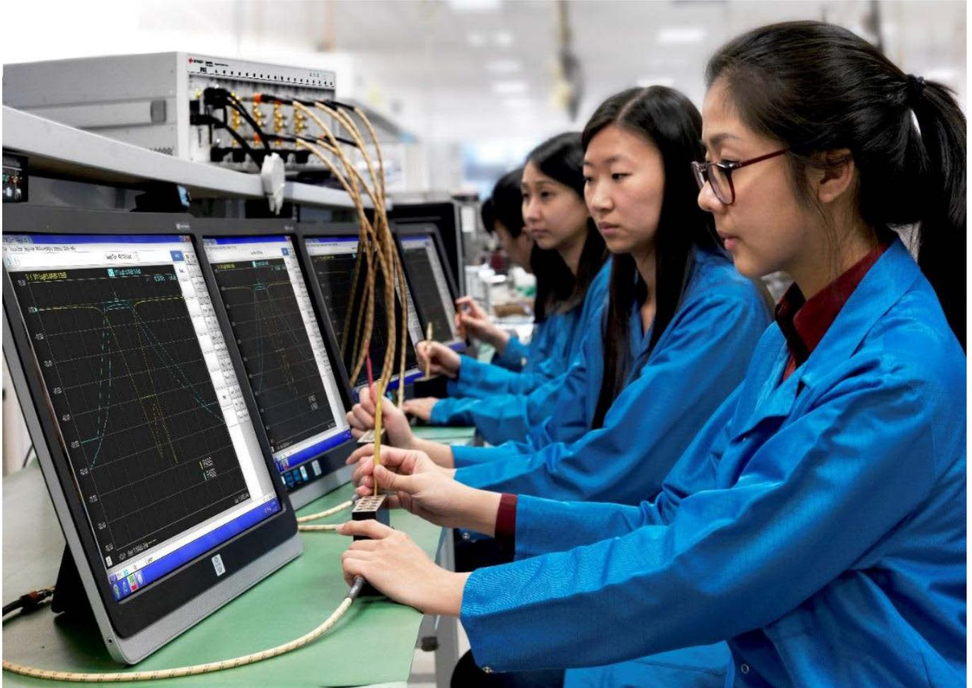
**Figure 1.** Tuning 4 independent filters using the multi-site configuration with multi-user and multi-display
