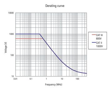
Probe derating curve (frequency limits measurable voltage) when used with ground spring tip
