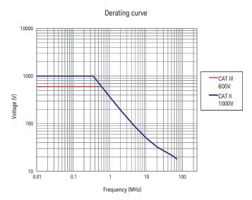
Probe derating curve (frequency limits measurable voltage) when used with the retractable hook tip
