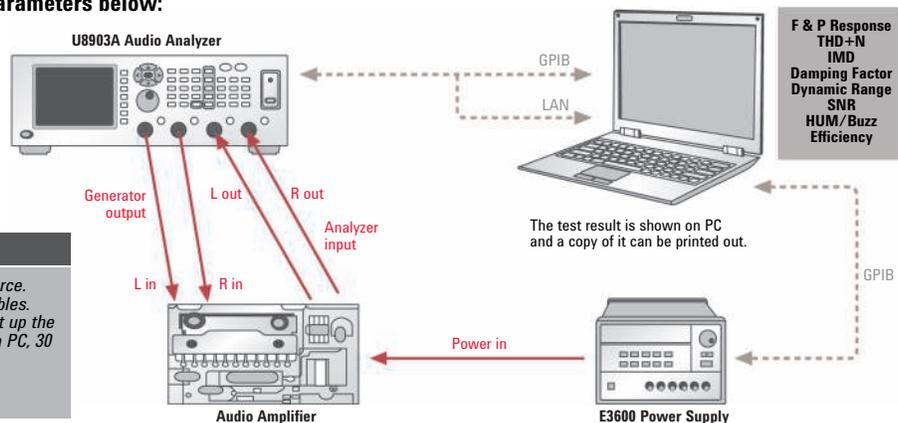
The test result is shown on PC and a copy of it can be printed out.
