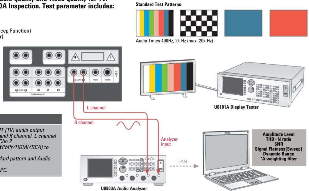
The test result is shown on PC and a copy of it can be printed out.
