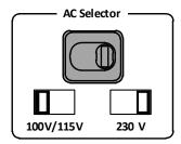
Figure 2-1 Orientation of voltage selector for different voltage selection
